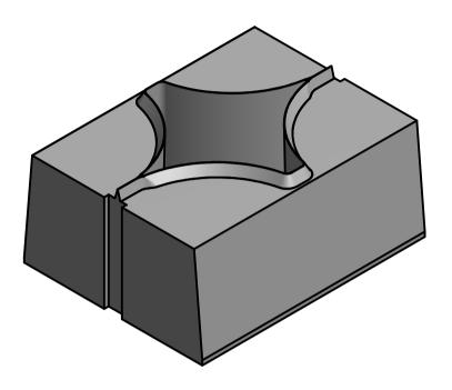
FS5040-3T FULL STAR R20,00 50x40mm, 23,70mm HIGH WITH 5° TAPERED SIDES TO SUIT 4mm CUTTING RULE
